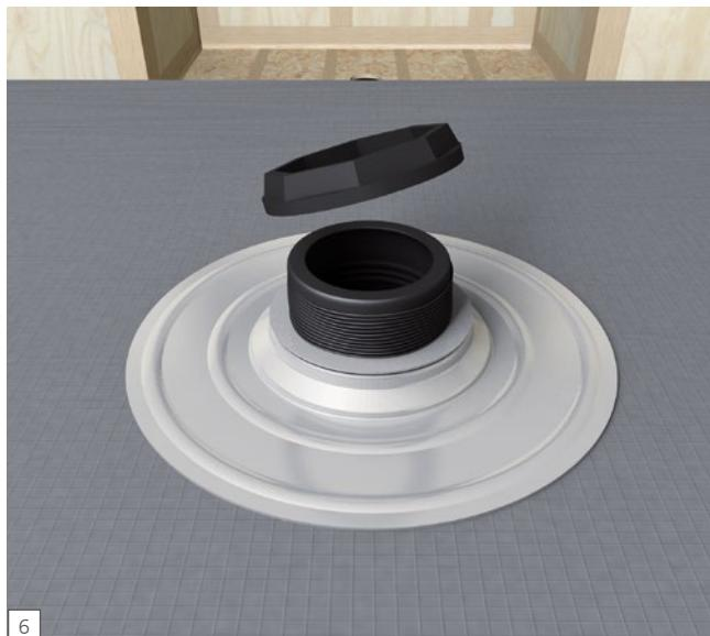
[EN] Tighten the gaskets firmly to the bases' steel ring using the locking nut. Make sure the drain body is still safely received in the valve-bead of sealant. Smooth out excess sealant over the drain body's flange surface.
